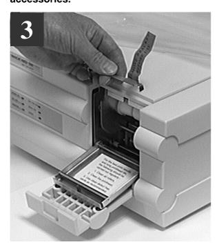
Open the front door and remove the metal shipping clip from the chassis.
